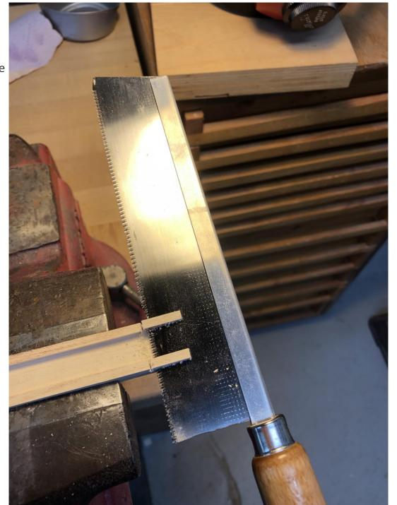
Dovetail piece with excess part of 5/8" block cut off with flush-cut saw.
